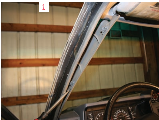
1. The OE pillar cover comes off easily with a screwdriver. Slip in under the edge of the cover, slide it down until you find the snap lock and carefully pry apart; then slide down to the next snap lock and repeat. Once you have the two snap locks free, simply lift and remove the OE pillar cover.
