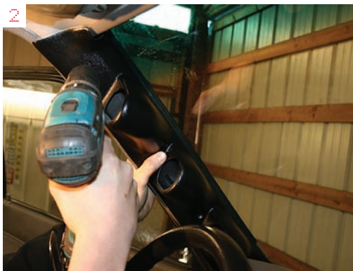
2. Hold the Truck Pillar into place, then use a 1/8" drill bit to slide in through the Truck Pillar's mounting holes and carefully spin the drill a couple revolutions to mark the A-pillar. Remove the Truck Pillar and drill the two holes.
