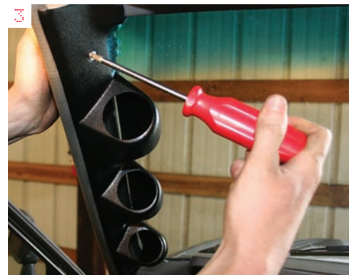
3. For a trial run we held the Truck Pillar back into place and ran in the supplied mounting screws. Everything fit up just fine so we pulled them back off to wire in the Glow Shift gauges.
